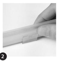
Position KKLN-01 Lens in clips by opening clip and inserting fully (10mm/0.39" max. gap between lenses for even linear illumination).
